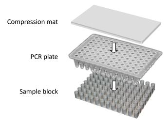
4. In order to prevent the deformation of the PCR vessels, and to ensure even distribution of the pressure from the lid, when PCR tubes or tube-strips are used, please load extra empty tubes on the 4 corners of the sample block. Always make sure that all the sample tubes/ tube-strips are distributed evenly on the sample block.
