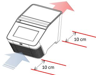
Please make sure there is no obstacle in the air flow path. At least 10 cm of space is required at the front and the back of the instrument.
